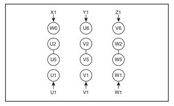
Figure 55. 440V motor wiring.
